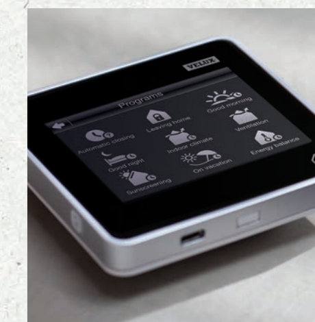
One remote control handles all skylights and blinds. Everything is solar powered - a must when you're off the grid.
